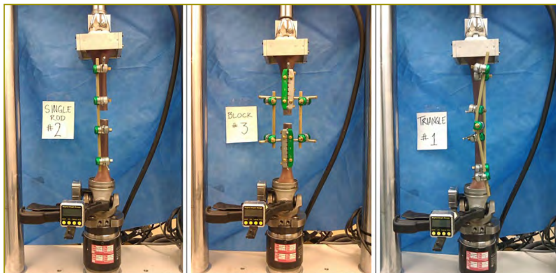
Figure 2. External fixation constructs tested in experimental study (aim 2). (Left) Single-rod uniplanar. (Middle) Pin-clamp uniplanar. (Right) Triangular two-planar. A total-knee prosthesis was used to simulate tibial-femoral articulation. A universal joint was used to simulate the ankle and subtalar joints distally.
