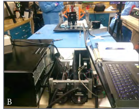
Figure 9. (A) Example of the device in active pronation/supination configuration. Yellow arrows show line of action of pull of the pronator teres and biceps brachii tendons during loading. (B) Placement of the linear motor system proximal to the baseplate to apply loads to the tendons while keeping the motor and associated electronic hardware clean from the cadaver testing.
