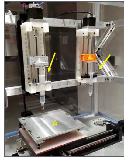
Figure 3. Close-up view of an early embodiment of our hybrid system showing the build plate (asterisk), bioprinter syringe pump (left arrow), and electrospinner syringe pump (right arrow).
