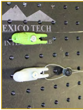
Figure 2. 3D-printed distal phalange undergoing uniaxial tensile testing to evaluate failure strength at the proximal interphalangeal joint of the prosthetic.
